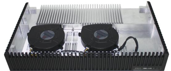
*Optimal thermal management design uses a combination of convection and conduction cooling to protect internal COTS components.*
